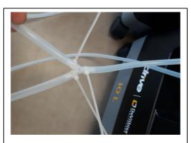
Tubing from the NRM can be plugged into the Y-piece. Concentrators are connected with either the silicone tubing 5mm (SCTDTUBE052) or with the standard tubing that comes with each face mask. The tubing should be secured onto the Y-piece
